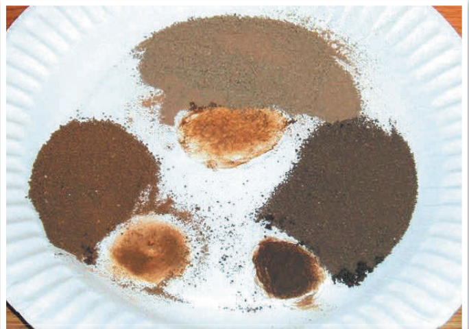
Examples of the three types of soil separated by sieving which also show contrasting colours: dark brown, pale/chalky and red.
